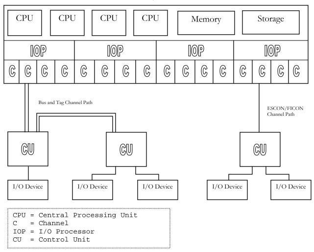
The 390 I/O systems come in 2 flavors the current 390 machines support both the older 360 and 370 interface, sometimes called the parallel I/O interface, sometimes called Bus-and Tag and sometimes Original Equipment Manufacturers Interface (OEMI).
