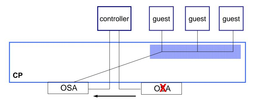
• If OSA dies or stalls, controller will detect it and switch to backup OSA
