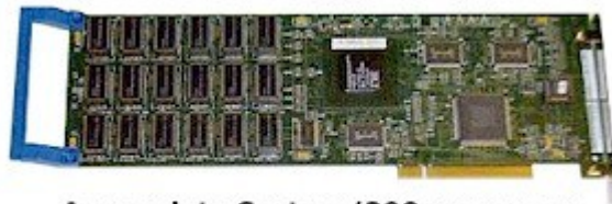
A complete System/390 processor on a single PCI card.
