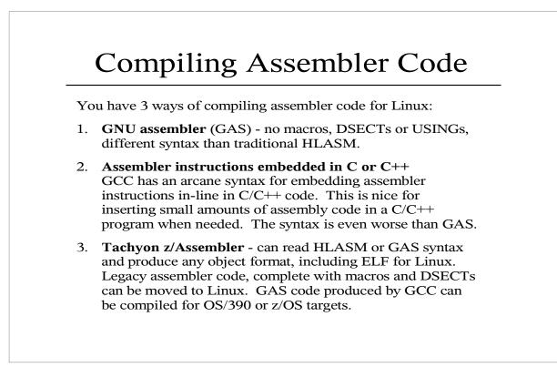
GCC produces GAS code, normally in a temporary file, before invoking the assembler to produce object code. Embedding assembler statements in C/C++ code causes those statements to be generated in the file sent to the assembler.
