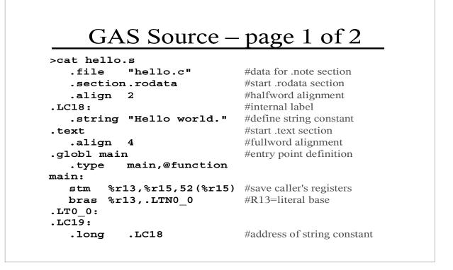
This is the 31-bit GNU assembler code produced by GCC 3.02 for Linux for S/390. The comments generated by GCC are omitted. The comments to the right of the GNU assembler code were added by hand.
