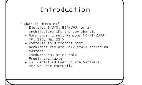
Hercules emulates the hardware of an IBM mainframe system. It doesn't provide any software services at all, any more than the bare iron does. You have to run some sort of OS on it.
