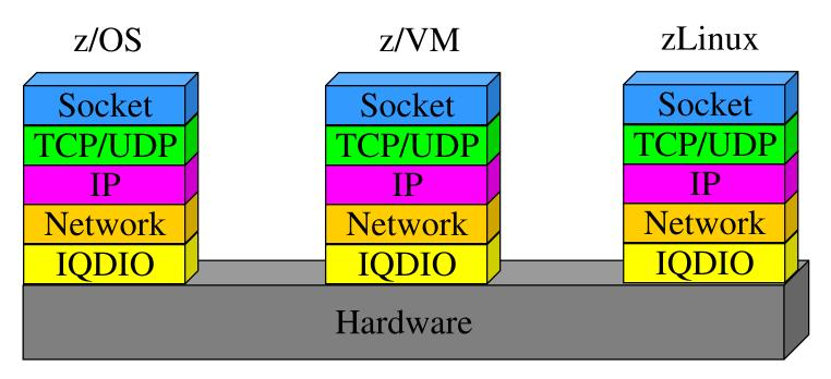
4 Virtual CHPIDs create 4 possible "virtual LANs" Not bound to a Plex Point to point routing
