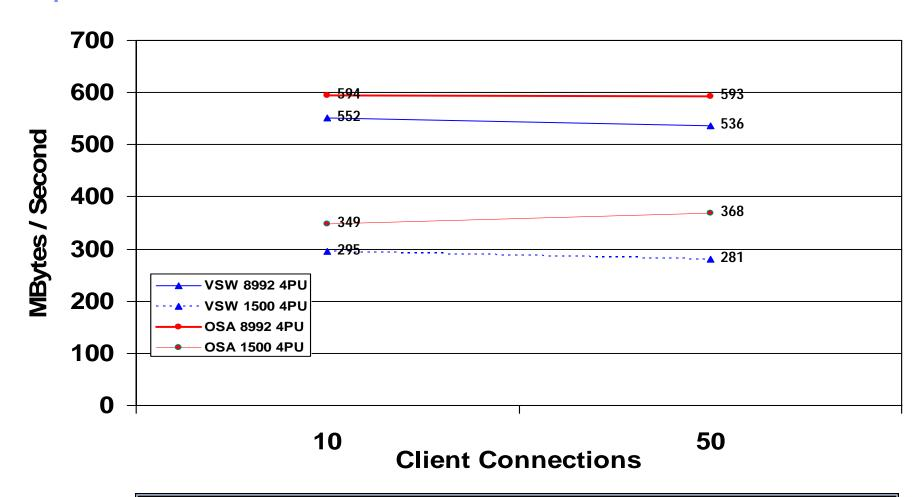
Using jumbo frames increases throughput between 61% and 91%.
