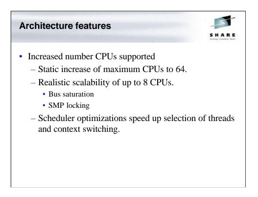
Linux 2.4 adds support for three new architectures: Intel ia64 (Itanium/Merced), IBM S/390, and Hitachi SuperH. (Intel Itanium/Merced CPU is not yet available.) Changes made to the 2.4 kernel are based on the current specifications and existing support for current 64-bit CPU architectures like the Alpha and Sparc64.
