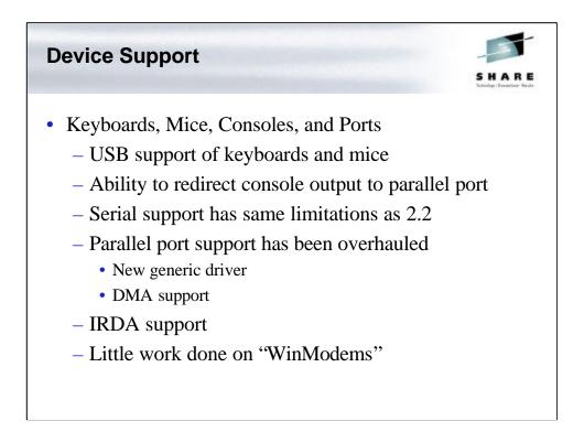
The biggest news on this front is that Linux 2.4 will support for the first time keyboards and mice attached to the Universal Serial Bus. When plugged in, these input device will behave just as if they were "normal" keyboards and mice. Additionally, Linux will now work on more systems, including broken (or specially embedded) ones where the keyboard is not pre-initialized by the BIOS. Also, better support is provided for machines without keyboards in some cases.
