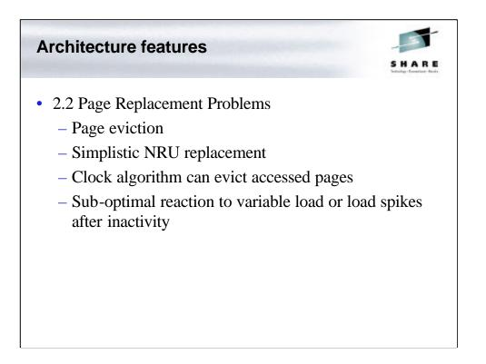
•Simple NRU replacement cannot accurately identify the working set versus incidentally accessed pages and can lead to extra page faults. This doesn't hurt noticeably for most workloads, but it makes a big difference in some workloads and can be fixed easily, mostly since the LFU replacement used in older Linux kernels is known to work.
