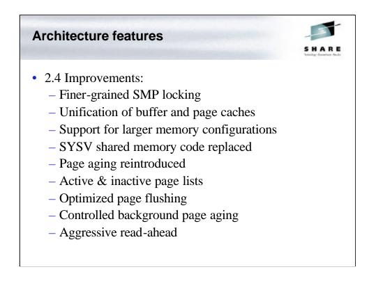
For Linux 2.4 a substantial development effort has gone into things like making the VM subsystem fully fine-grained for SMP systems and supporting machines with more than 1GB of RAM. Changes to the pageout code were done only in the last phase of development and are, because of that, somewhat conservative in nature and only employ known-good methods to deal with the problems that happened in the page replacement of the Linux 2.2 kernel.
